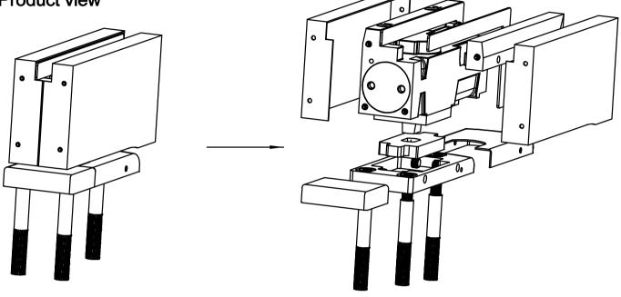
Keep the gaps as per drawing, make sure the top and bottom pivot center are well aligned.
